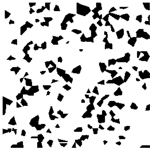
Fig. 1. An example simulation lattice generated by a Voronoi tessellation of the plane with \phi = 0.5 . Black regions represented the dispersed metal particles and white regions the catalyst support.
